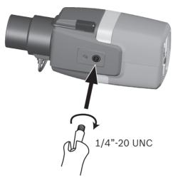
Figure 5.2 Mounting a camera
